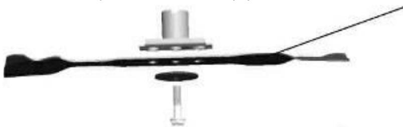
Replace everything as shown. Fasten the screw properly. Fastening torque is 45Nm. Also, replace the blade screw when replacing the blade.
