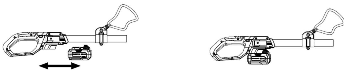
Figure 4: Installing the battery
