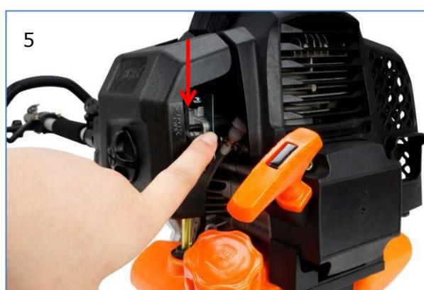
5. **Necessary:** Set the choke lever to the "WARM START" position after the engine has responded and immediately pull the starter again until the engine starts. " see also video device start on our homepage."
