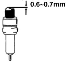
5 Check the spark plug washer and screw the spark plug in the first 2-3 threads manually first.
