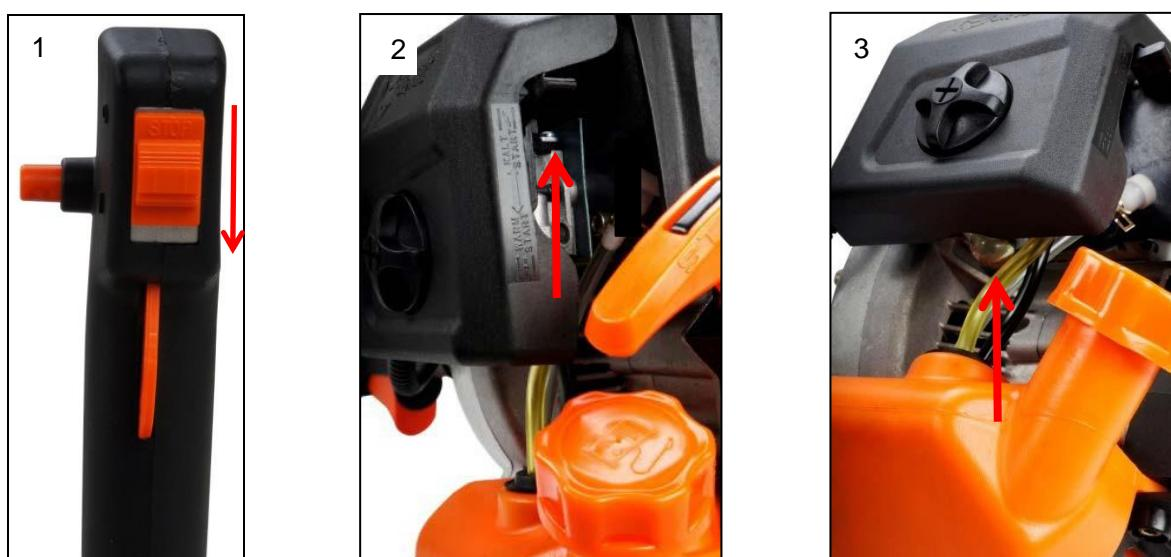
2. Move the choke lever upwards to "COLD START."
