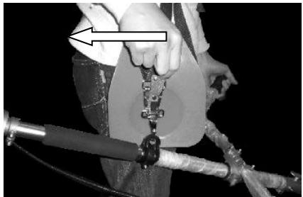
The shoulder strap is equipped with a quick-release device (see picture). You can quickly remove the shoulder strap by pulling the quick release.
