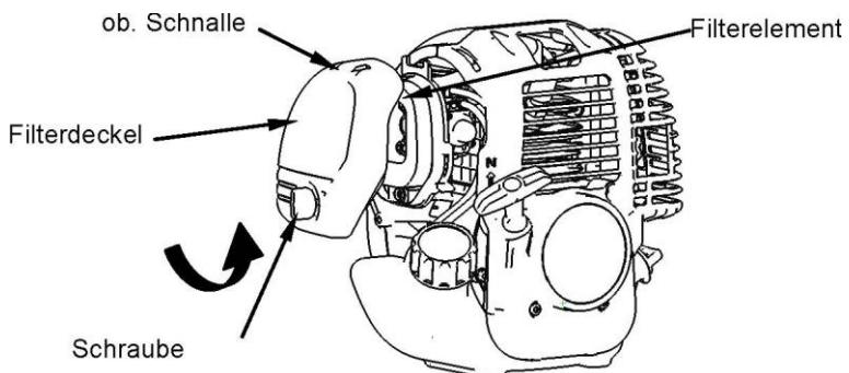
2 Use non-flammable solvents or cleaning agents with a high flashpoint to clean the filter element and let it dry completely.
