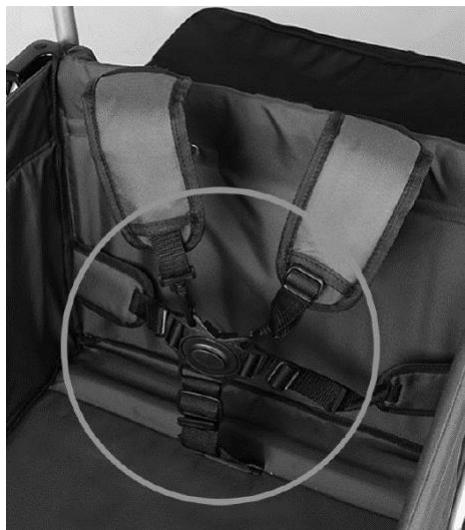
Insert the combined shoulder belt/pelvis belt buckles into the buckle to close the 5-point safety belt.
