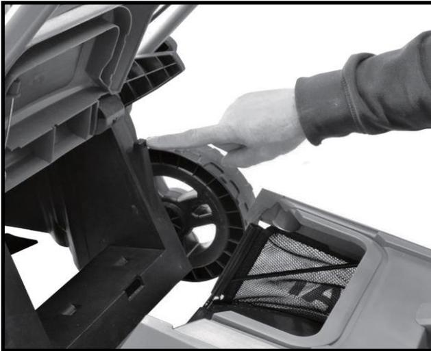
To install the grass catcher basket on the mower, lift the tailgate and attach the basket.
