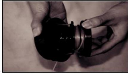
5. Remove the excess thread.
