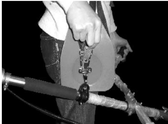
The shoulder strap is equipped with a quick-release device (see picture). You can quickly remove the shoulder strap by pulling on the quick-release device.
